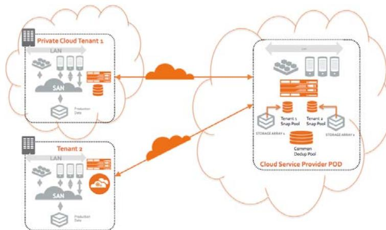
**Figure 5 Data Storage Isolation with Actifio VDP**
